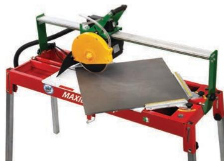
Suitable for cutting porcelain, ceramic, marble and granite tiles. Special voltage ratings available. Direct drive. Cutoff switch with thermal cutout (a). Cooling by water pump and flow governor cock (b). Motor unit slides on four adjustable iron pulleys (c). 45° jolly cuts (d). Swinging head can be locked at the desired height (e). Square for linear and diagonal cuts (f). Support square for diagonal cuts. Side extension for big tiles (g). Cutting table width cm 115 x 45 (45" x 18").
